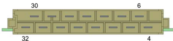
CONECTOR / CONNECTOR DIN 41612 H15 - Max. 12A / Terminal
